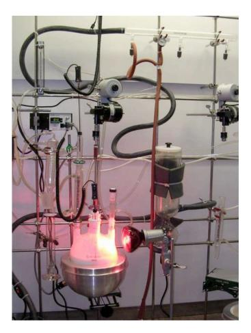
The resulting lab resin is discharged in molten form. It is then cooled and crushed to prepare it for use in a typical thermosetting polyester powder coating formulation.
